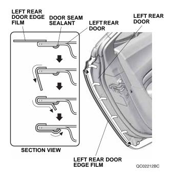
22. Using a shop towel, wipe off any excess tape application solution from the door. Allow the door edge film to dry thoroughly.
