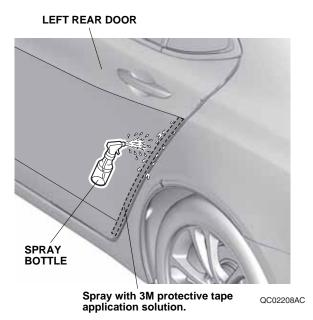
17. Open the left rear door. Peel back about 50 mm (2.0 in.) of adhesive backing from the left rear door edge film. Align the top edge of the protective film with the bottom of the character line, and the V-notch with the door edge.
