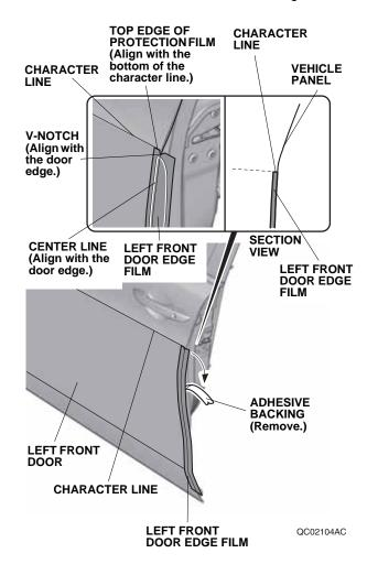
Align the center line on the left front door edge film with the door edge. While applying light pressure, carefully remove the adhesive backing. Go to step 12.
