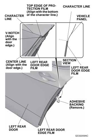
18. Align the center line on the left rear door edge film to the door edge. While applying light pressure, carefully remove the adhesive backing.
