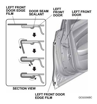
15. Using a shop towel, wipe off any excess tape application solution from the left front door. Allow the film to dry thoroughly.
