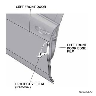
14. Starting from the center and working outward, use your fingers to fold the door edge film inside the door. Move your fingers in one direction only. Do not damage the door seam sealant.
